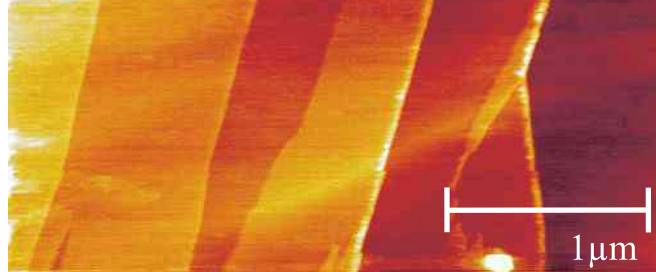
Figure 7.2: Bi 2 Te 3 surface image. Atomic force microscopy image of an exfoliated Bi 2 Te 3 surface. The step edges are 1.0 nm high, corresponding to the Bi 2 Te 3 quintuple unit cell. These nanometer flat surfaces span an area up to 50 × 50 μm 2 .
